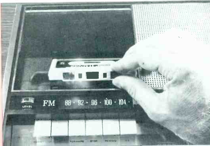
Fig. 2. Cartridge goes into machine rear-first. Leaf spring behind cartridge snaps it into place as front is pushed down.
