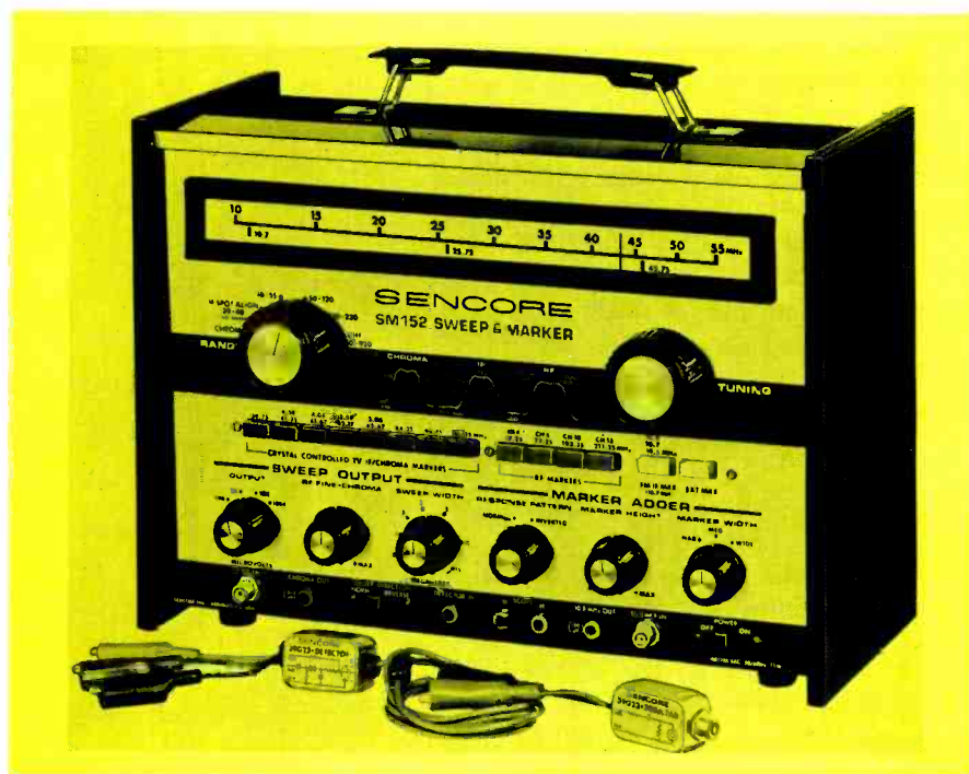
Fig. 1. With modern equipment, such as the Sencore unit shown here, sweep alignment is much simpler than in the old days, when it took many instruments and a couple dozen connections to get hooked up and ready to view a response curve.
